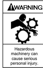
**Failure to disconnect and lockout electrical power or engine drive before attempting maintenance can cause severe personal injury or death**
