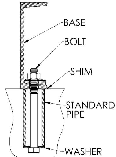
**Figure 3 - Anchor Bolt**
