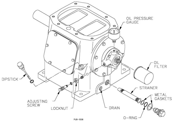
**Figure 6 - Compressor Lubrication System**
