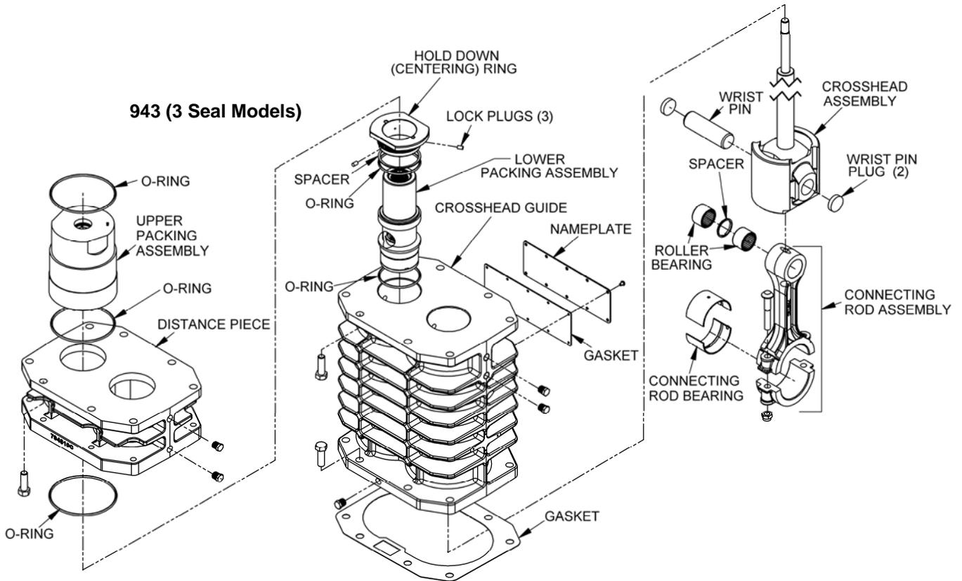
Figure 8 - Packing Boxes, Crosshead and Connecting Rod Detail
