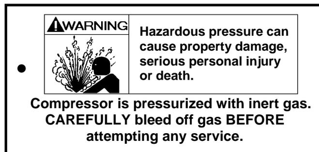
Figure 23 – Pressurized Compressor Tag
