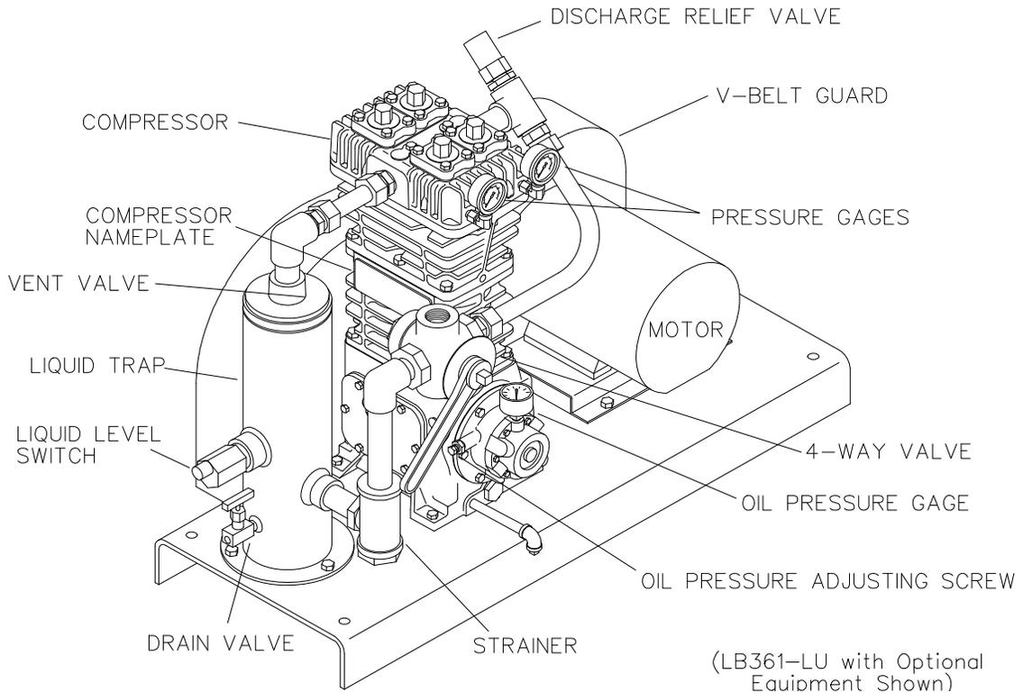
**Figure 6 - Typical Liquefied Gas Transfer Compressor**
