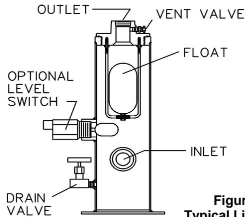
**Figure 7 – Typical Liquid Trap**
