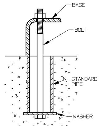
**Figure 3 - Anchor Bolt**
