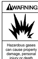
**Extreme temperatures caused by abnormally high discharge pressure or valve problems can be a source of ignition in explosive atmospheres causing severe personal injury or death.**
