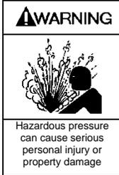
Failure to relieve system pressure prior to performing compressor service or maintenance can cause serious personal injury or property damage.
