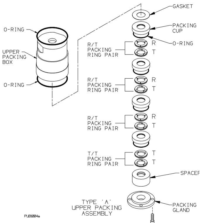
**Figure 14 - Upper Packing Assembly -LB942
