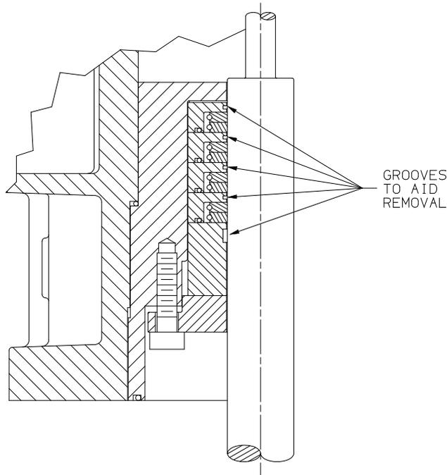
**Figure 15 - Upper Packing Section View – LB942
