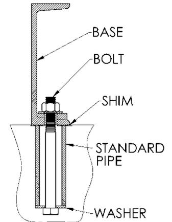
**Figure 3 - Anchor Bolt**
