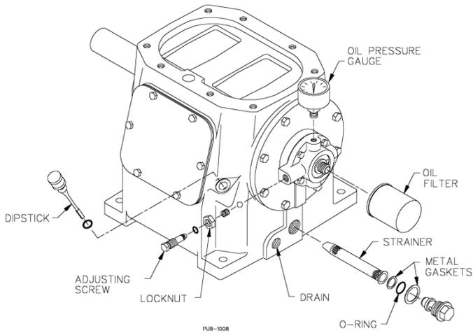
**Figure 9 - Compressor Lubrication**
