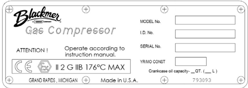
**Figure 2 - Compressor Nameplate**
