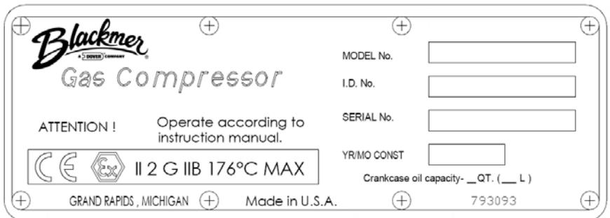
**Figure 2 - Compressor Nameplate**
