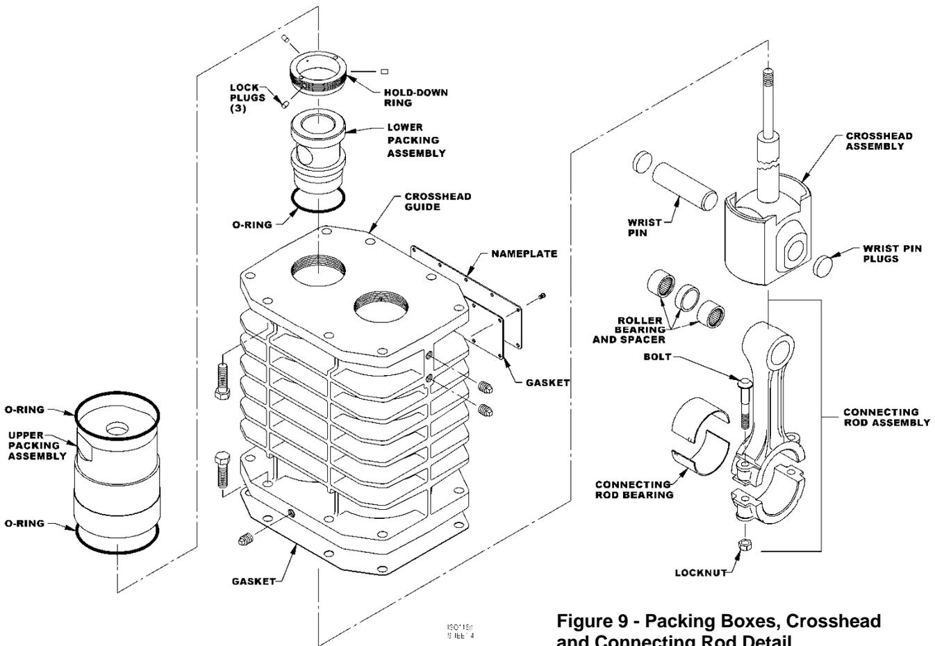
**Figure 9 - Packing Boxes, Crosshead and Connecting Rod Detail**
