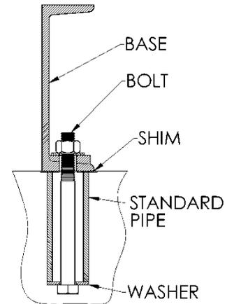
Figure 3 - Anchor Bolt
